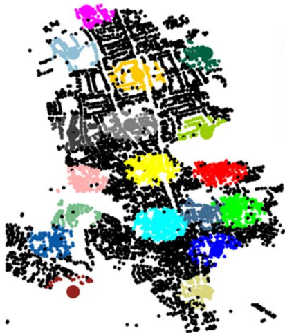
Fig 4: Coverage planning when threshold is at -70 dBm and BS power is at 20dBm
