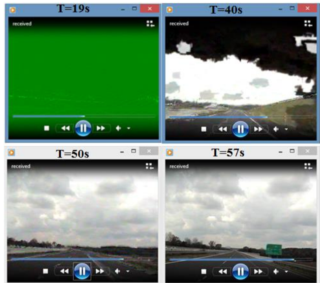
Fig. 9: screen captures of the video received across a network topology of D = 100m, N=64 nodes, DSDV protocol
